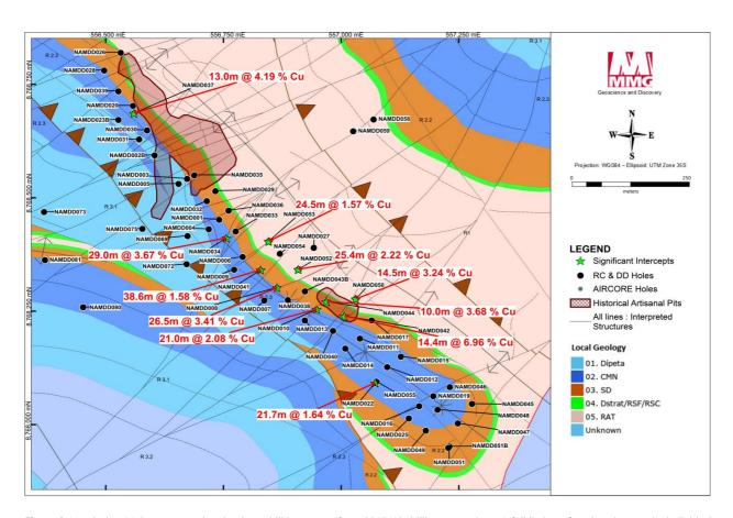
Figure 9: Nambulwa Main prospect showing best drill intercepts from 2017/18 drilling campaigns. A full listing of exploration results in Table 2.
