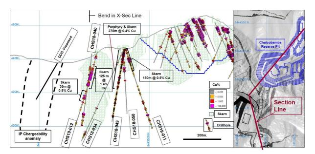
Figure 7. Cross Section drawn through the Chalcobamba Resource/Reserve Pit and the adjacent Chalcobamba Southwest Zone (left) highlighting the individual drillhole traces, downhole copper assays as well as individual mineralized intervals. Skarn polygons are shown as hatched green area.
