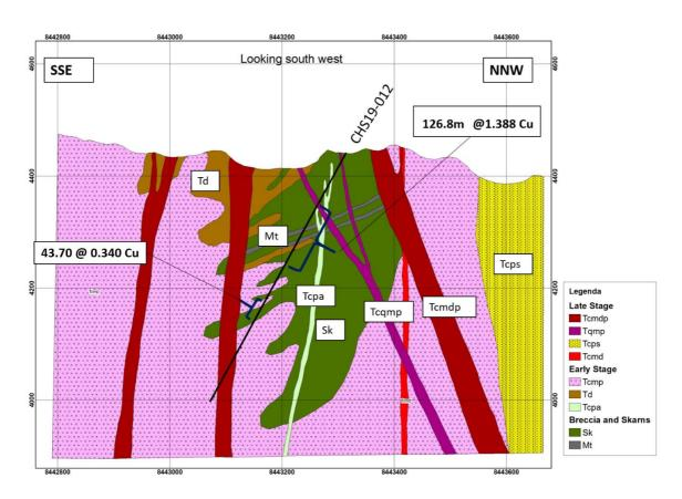
Figure 4. Geologic Cross Section through drill hole CHS19-012. Refer to Figure 2 for drillhole location.
