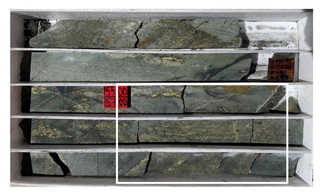
**Figure 5.** Strongly disseminated chalcopyrite mineralisation hosted by skarn alteration within diamond drillhole CHS19-012. Core box contain half core from 152.75m to 155.70m. Rectangular white outline defines area of close-up photograph shown in Figure 6 below.
