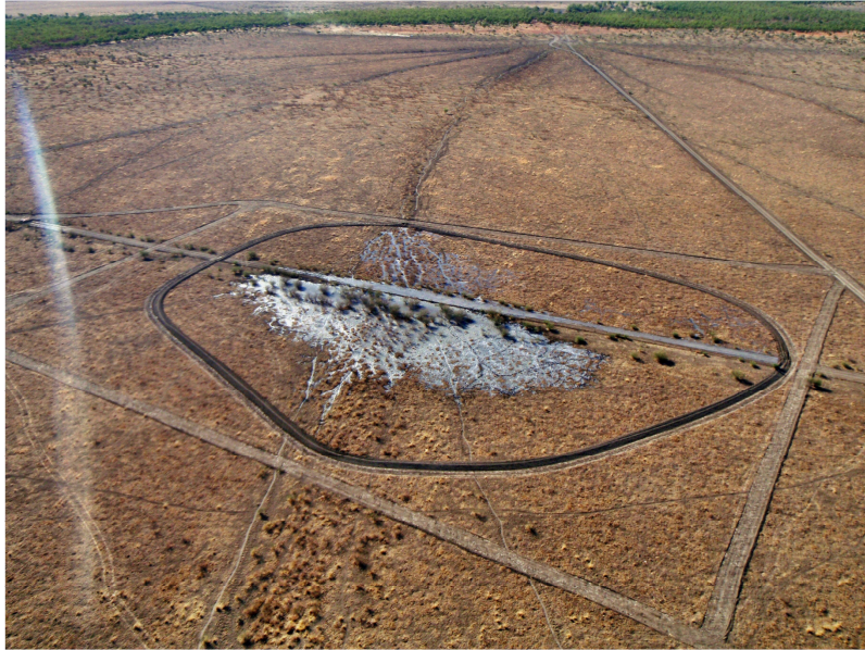
Aerial view of spill with fence and bund.
