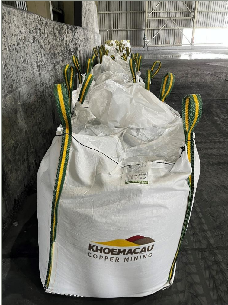
Figure 13-18 Two-tonne Bulka Bags ready for transport
